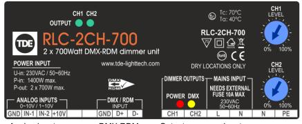
Analog inputs DMX-RDM Output power Input power
