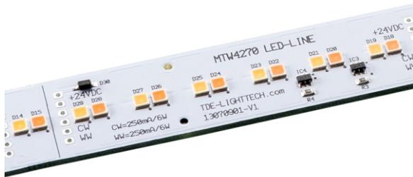
The MTW4270 is a tunable white LED module that is capable of changing its colour temperature from 4000K to 2400K. This allows the user to create a dynamic ambience with the extra warm 2400K colour temperature as a unique feature.
