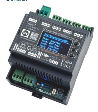
The IZI-SplitterMerger+RDM is the next evolution in smart DMX management. It combines a robust DMX splitter and a powerful merger in a single compact module. With two inputs (one doubling as an output in splitter mode) and four dedicated outputs, the module delivers five outputs in splitter mode or four in merger mode. Whether you need LTP, HTP, or backup merge modes, this device is ready for any professional lighting setup.
