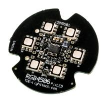
The RGB4506 is a modulair LED pixel system, a solid-state design with six high intense RGB LED's. With an ultra-high visual refresh rate (patented technology) this led module is extremely suitable for studio applications.
