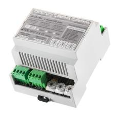
The AD-LC6 MKII is a high power 6 channel LED driver. This versatile LED driver can be used for our RGB, single colour and tunable white LED modules as well as our LED spot range . The driver is controllable through DMX-512 but also offers stand-alone functions and is configurable with its internally selectable user modes. The refresh rate of this driver is adjustable up to 1800Hz which makes this driver suitable for studio applications.
