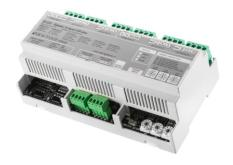
The AD-LC12 is a high power 12 channel LED driver. This versatile LED driver can be used for our RGB, single colour and tunable white LED modules as well as our LED spot range . The driver is controllable through DMX-512 but also offers stand-alone functions and is configurable with its internally selectable user modes. The refresh rate of this driver is adjustable up to 1800Hz which makes this driver suitable for studio applications.
